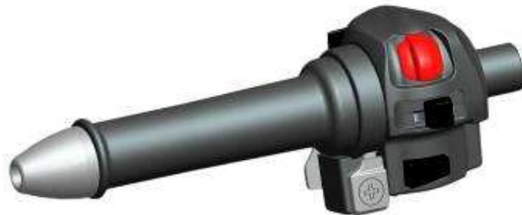
It is **adjustable on 8 levels** even **when riding** even with the **throttle open** thanks to a **joystick** on the left handlebar:
